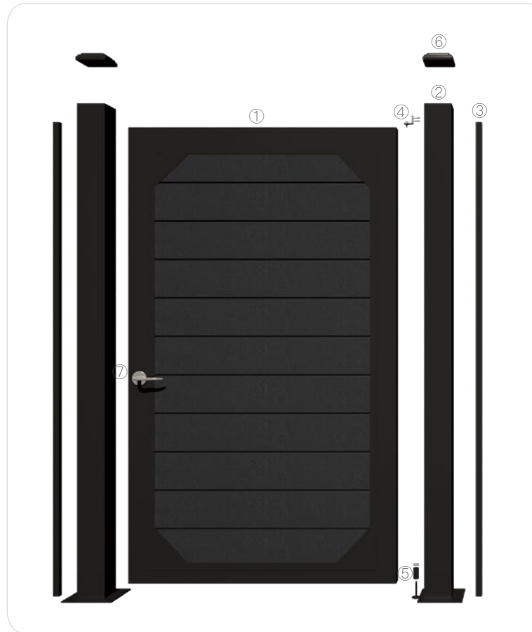
① Fence Gate CWB-01(1665x900mm)
